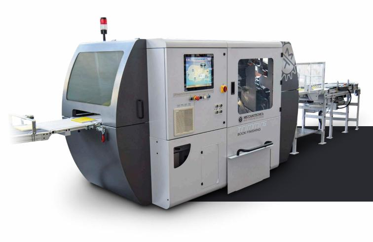
**Trimming**, the automatic three-knife trimmer performs fully variable changeovers producing books in short runs, down to one copy, even with flaps.
